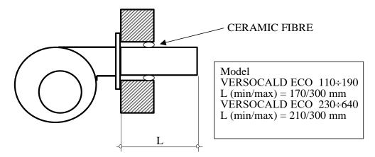
Secure the burner to the door by means of the fixing plate so that the flame is parallel and centred in the furnace; if not, combustion problems can occur with the risk of seriously damaging the boiler.
